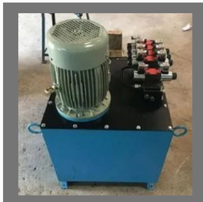
Hydraulic Power Pack
